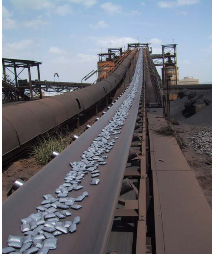
FINMET® Production to Shipping Silos
