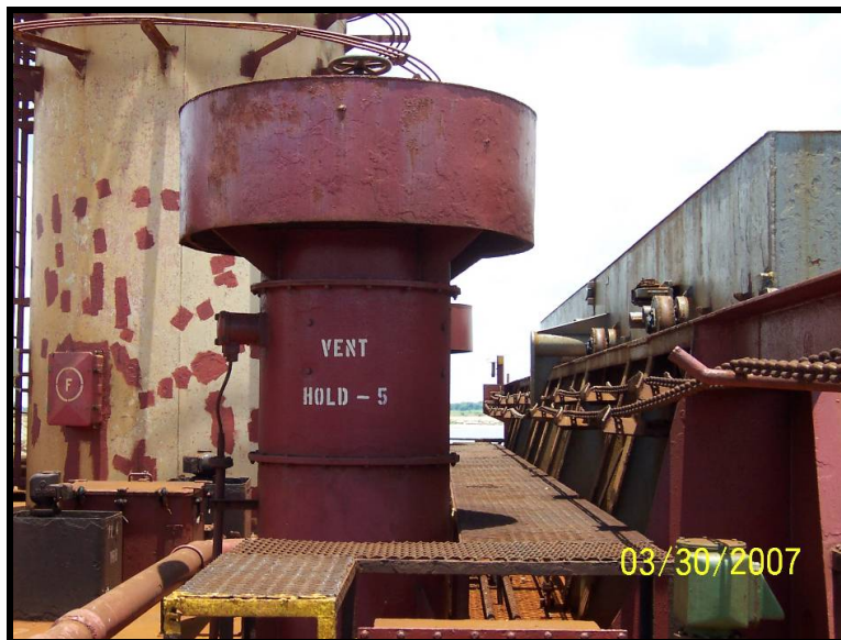
Figure 10 - Mechanical ventilation device on hatch covers
