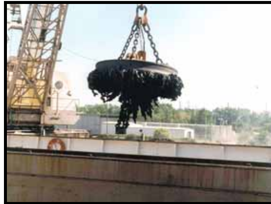
Figure 18 – Handling HBI with a magnet
