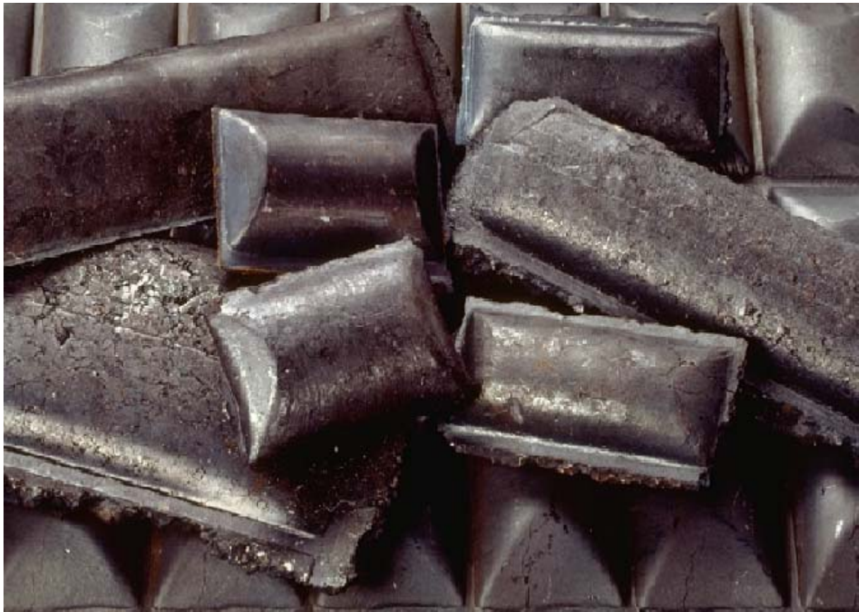
Figure 2: HBI Briquettes with different shapes and volumes
