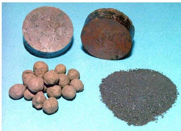
Figure 3: DRI samples from pellets and fine ore and corresponding compacts produced in the punch and die press
