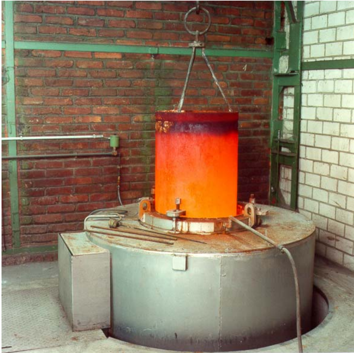
Figure 6: Electrically heated furnace at KÖPPERN's test facility during the extraction of a hot test sample.
