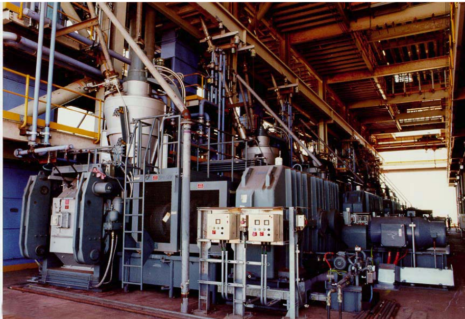
Figure 3: Briquetting machine for the production of HBI from fine ore, roller diameter 1,400 mm
